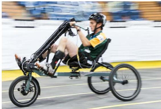
Pilots with complete paraplegia ride in a bike race using functional electrical stimulation of their muscles. The nerve pathways controlling these competitors' leg muscles are interrupted. By externally attaching electrodes to the legs, it is possible to send electrical impulses to the muscles, thereby causing the muscles to contract. The pilots can often stimulate the muscles themselves using a controller.
