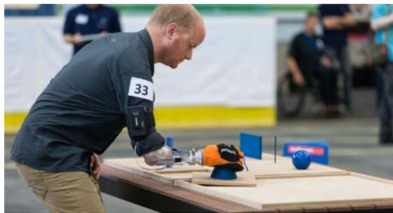
Pilots with upper-arm amputations use motorised arm prostheses to complete physical challenges quickly and with precision.
